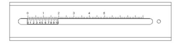
Figure 3. Delay length change ruler for the F-VDL device. The marked unit in the stationary scale is in centimeters with millimeter subdivisions.
