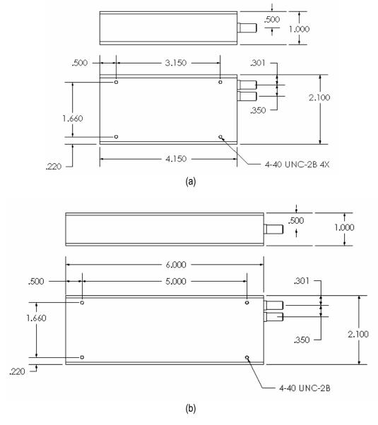
Figure 2. Mechanical layout of the F-VDL manually variable optical delay line: (a) 330 ps model, and (b) 600 ps model
